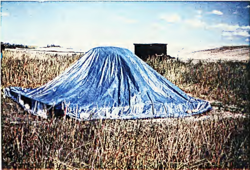
Figure 5.2 Lysimeter was Covered to Prevent Rainfall Inputs and Evapotranspiration Losses during the Experiment. Garbage Bin (in background) Supplied the Irrigation Water for the Tests
